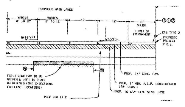
18. In addition, TxDOT erected a precast concrete barrier ("CTB TYPE 2") in the median between the east/west lanes of IH-10. The barrier was installed in sections thirty feet (30') long, each weighing approximately seven (7) tons and rising thirty-two inches (32") above the now-elevated grade level of the traffic lanes. And, importantly, the 30-foot sections are grouted together so as to form a complete seal.
