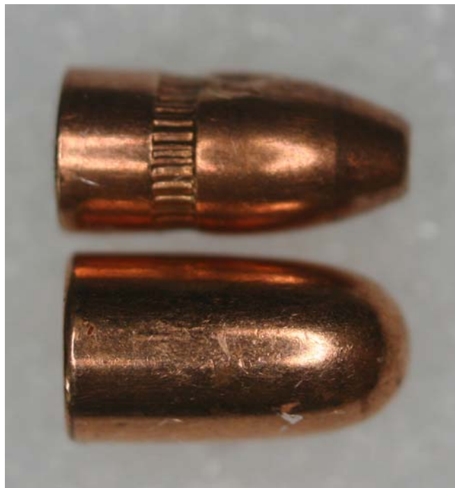
IMAGE 2: Unfired .22 Magnum rimfire caliber bullet (top) compared to a .25 auto caliber bullet (bottom)
