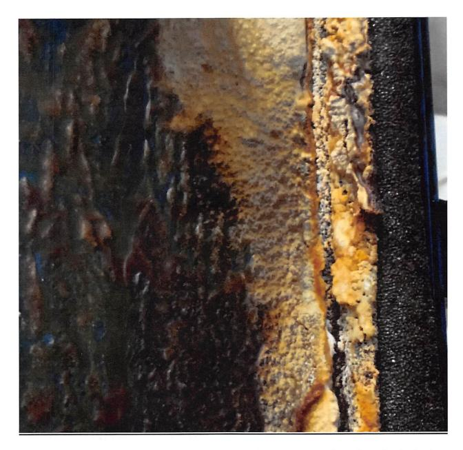
67. The growth of mold in the dust collection system and throughout the Packaging Suites at Cleveland is unsurprising because SAFC did not have adequate cleaning and sanitation practices. Instead of carefully monitoring and documenting the sanitation and cleaning of the air filtration systems and the packaging rooms as required, SAFC Cleveland staff often sprayed down the Packaging Suites and equipment, including the air filters in the packaging rooms, with water.
