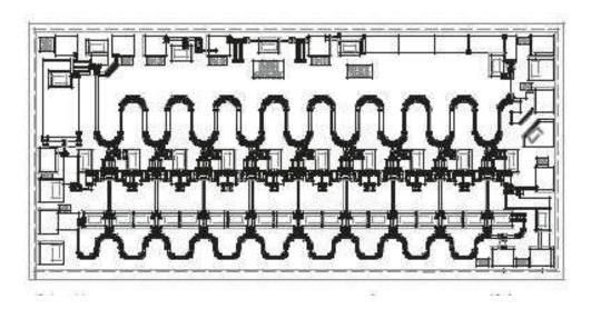
This basic apmlifier architecture is quite literally a "textbook" design; a microscope photograph of the corresponding chip (apparently manufactured at Agilent's facility in California) is featured
