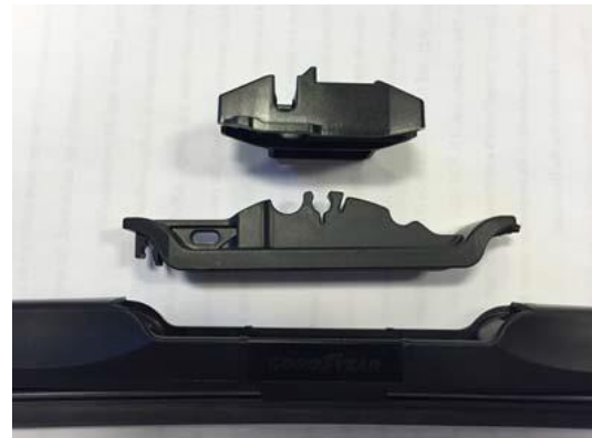
Goodyear Hybrid Connector Structures
