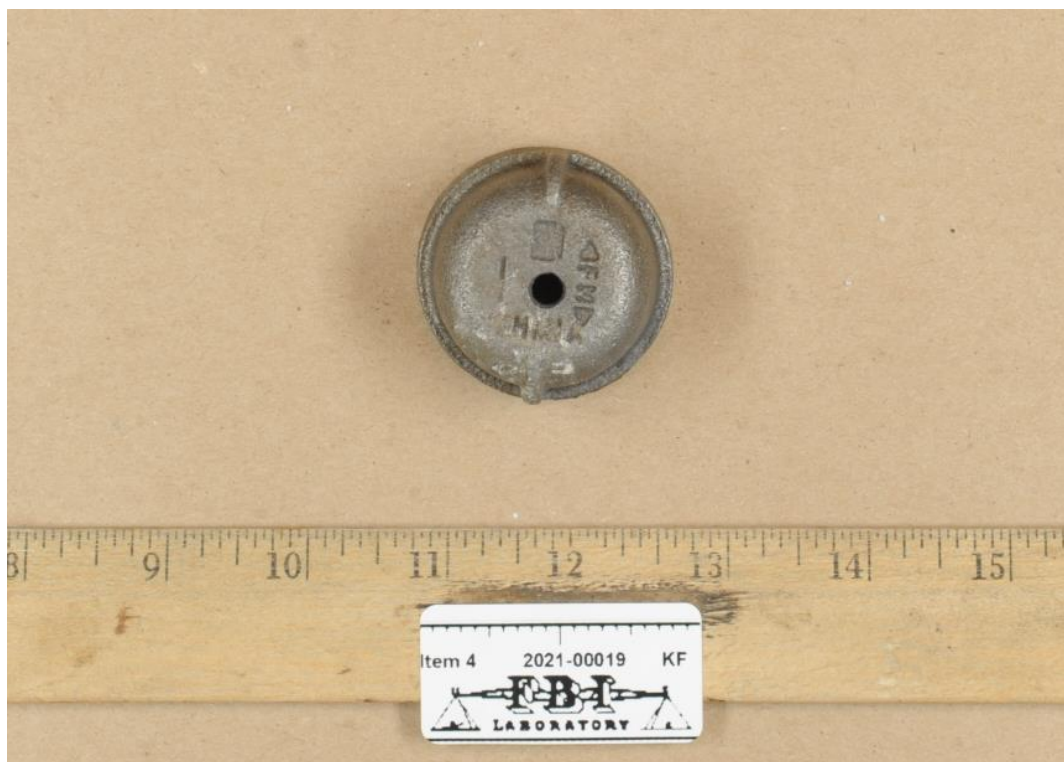
Figure 5 Item 4 One (1) end cap with priming hole.
