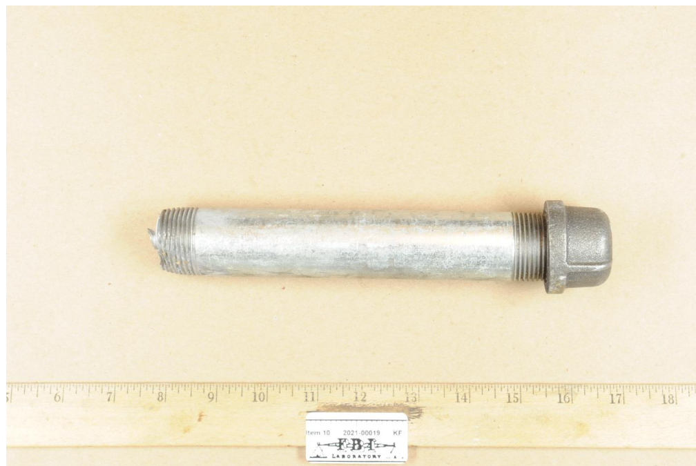
Figure 12 Item 10, Pipe nipple with solid end cap
