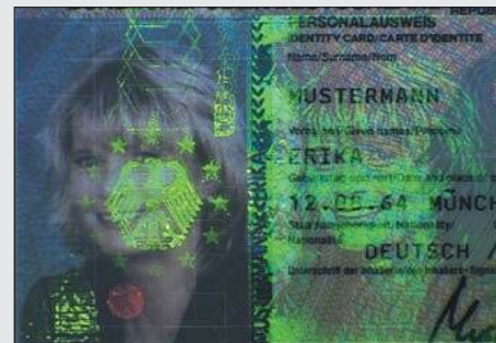
Below: OVDs revealed with LED illumination.
