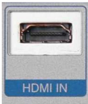
Figure 2: Image of HDMI socket on a display device. Source: Public Domain Image available at https://en.wikipedia.org/wiki/File:HDMI.socket.png
