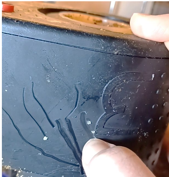
Figure 1: Degraded plastic on Plaintiff's coffee grinder
