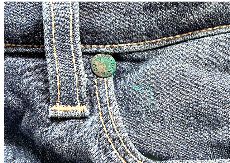
Figure 2: Chemical reaction to copper alloy on Plaintiff's jeans
