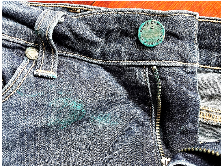
Figure 4: Chemical reaction to copper alloy on Plaintiff's jeans
