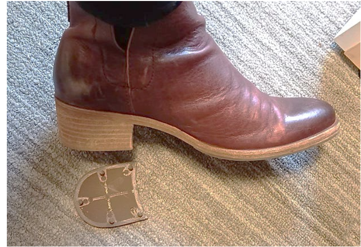
Figure 3: Plaintiff's shoe falling apart in use due to dissolved glues
