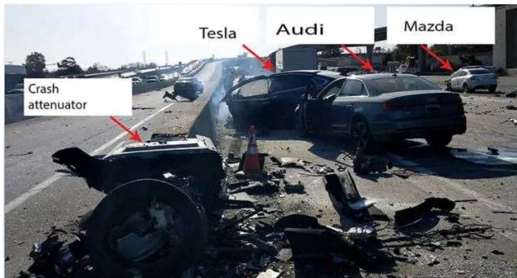
8 9 10 11 12 13 14 15 16 Fatal 2018 crash involving Autopilot, in which Tesla’s software suddenly steered the Tesla to the left, directly into a concrete barrier on a highway in Mountain View, California. Photograph by NTSB.
